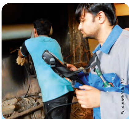
Understanding the current situation through measurement is an important step to determine the most effective RECP improvement required at SMEs. Here a RECP consultant is analysing the exhaust gases of a zinc melting furnace with the help of furnace operator at a pipe manufacturing company in Bangladesh.
