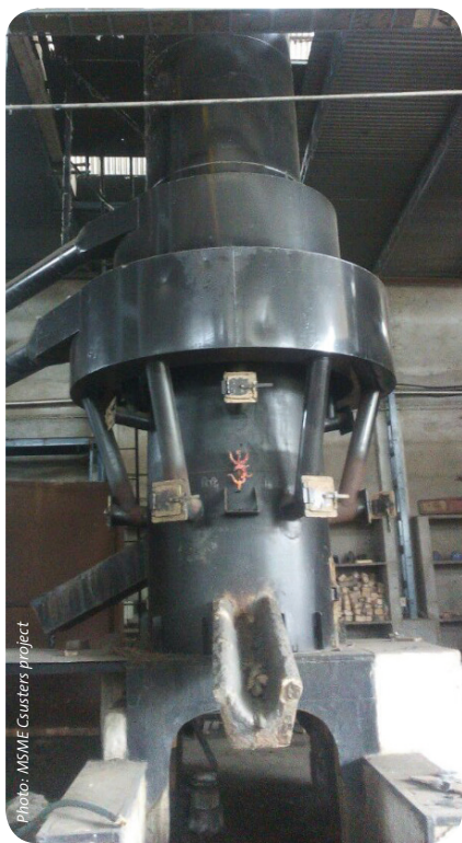
New divided blast cupola installed
